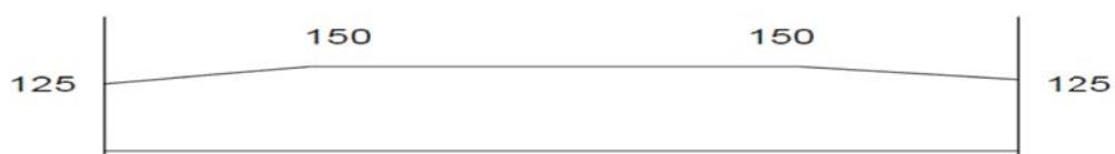
"Alternate End Stressing" results in symmetrical stresses due to prestress
